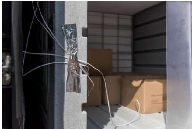
Figure 2. Temperature sensors in different points inside the Coldtainer
